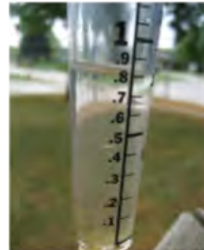
Rain Gauge Measures amount of precipitation
