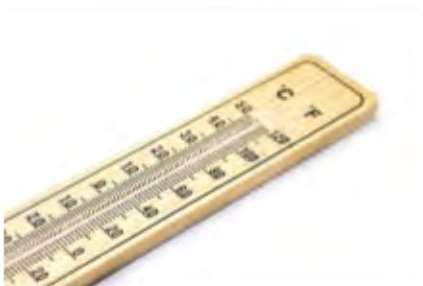
Thermometer Measures temperature
