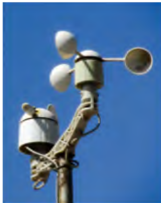
Anemometer Measures wind speed
